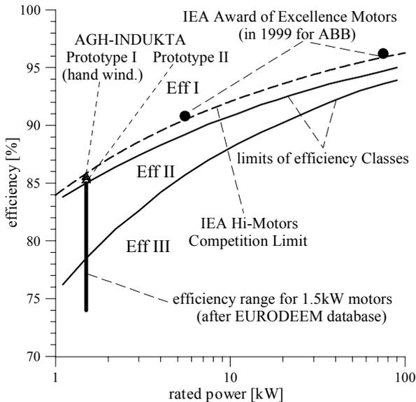
Fig.1. Results obtained for prototypes of the Class Eff I induction motor SEE90L-4 in comparison to the European Database of Efficient Electric Motors (EURODEEM)
