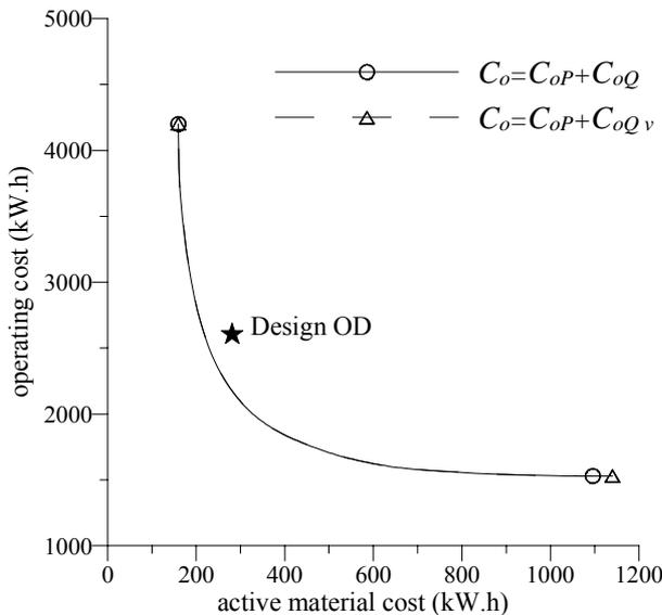
Fig.2 A comparison of cost functions for optimal designs for two cases (a) and (b) of the operation cost  $C_o$  in (9). Design OD is a design arising from (1) for Prototype II.
