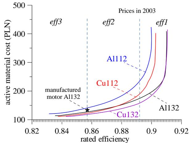
Fig. 5. Influence of rated efficiency on motor material cost. Price level in 2003 (1EUR=4.1PLN, 1US\$=3.95PLN)
