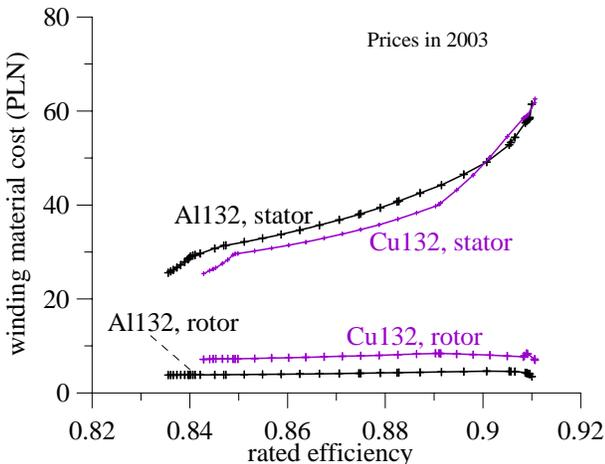
Fig. 8. A relationship between rated efficiency and cost components of “132” motor windings
