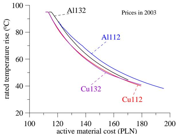
Fig. 6. Stator winding rated temperature rise as a function of active material cost for selected motor constructions.
