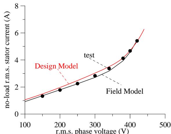
Fig. 3. No-load r.m.s. phase stator current from measurement (test), field calculations (Field Model), and analytical calculations (Design Model)
