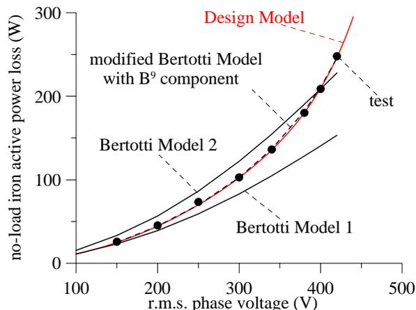
Fig. 4. No-load iron losses from measurement (test), field calculations (Bertotti Models), and analytical calculations (Design Model)
