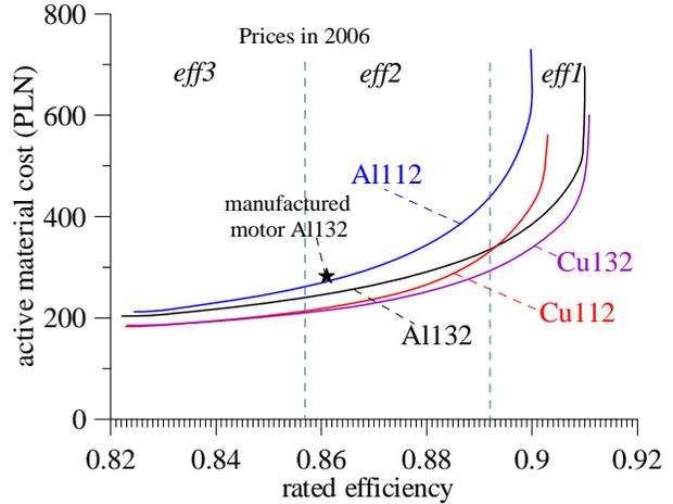
Fig. 9. Influence of rated efficiency on motor material cost. Price level in 2006 (1EUR=4.1PLN, 1US\$=3.2PLN)
