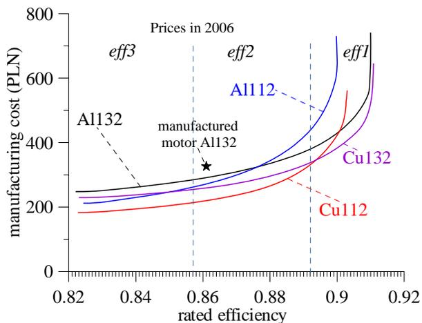
Fig. 12. Influence of other production cost components on relationship between manufacturing cost and rated efficiency.
