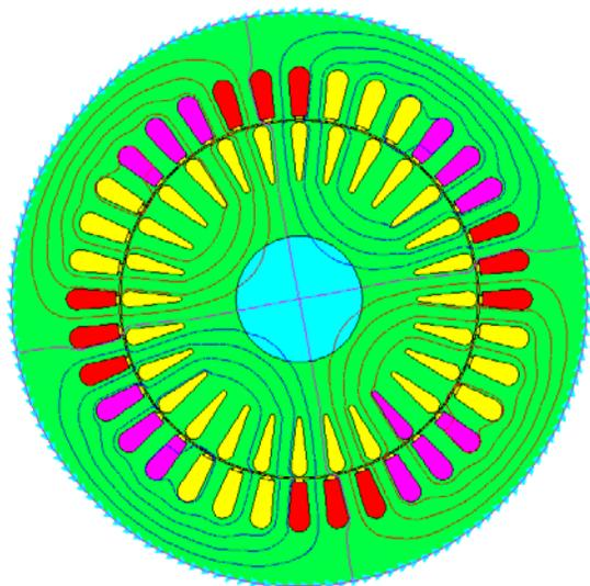
Fig. 2. Analyzed motor sheet geometry with equiflux lines at no-load.
