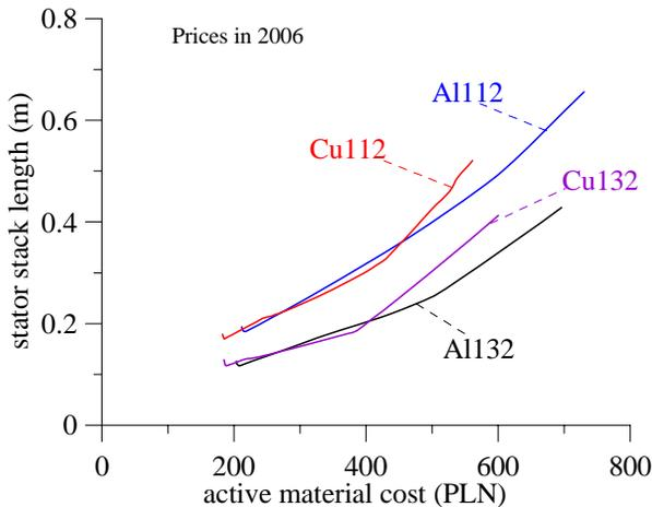
Fig. 11. Almost linear relationship between motor stack length and its active material cost for analyzed motors in an area of practical interest.
