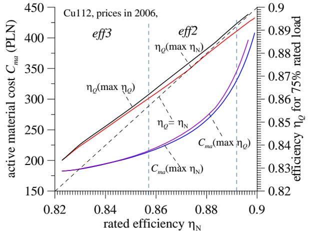
Fig. 10. A comparison of motors designed by a criterion  $\max \eta_N(P_N)$ , and  $\max \eta_Q(P_Q = 0.75P_N)$  for “Cu112” motors.
