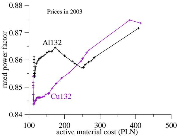
Fig. 7. A variation of rated power factor for “Al” and “Cu” motors as active material cost increases. Marked points denote solutions generated by solving algorithm.
